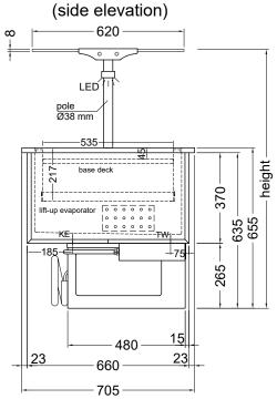
TW = Drain DNØ30 KE = Cooling/Electric
